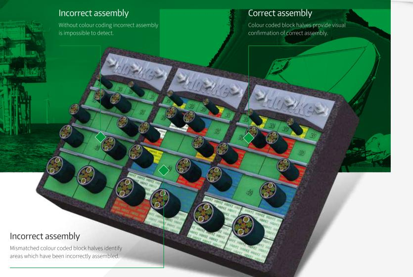
Stray signal/noise cannot pass through the conductive EMC and pass to earth. Tolerant and filler blocks have a cable range of 3 mm to 100 mm and are coated with a high conductive material. Copper tape provides high conductive path from cable screen to earth. Frame zinc plated or stainless steel to allow conductivity from blocks to earth. Simple preparation of cable and assembly of system without modification of insert blocks onsite.
